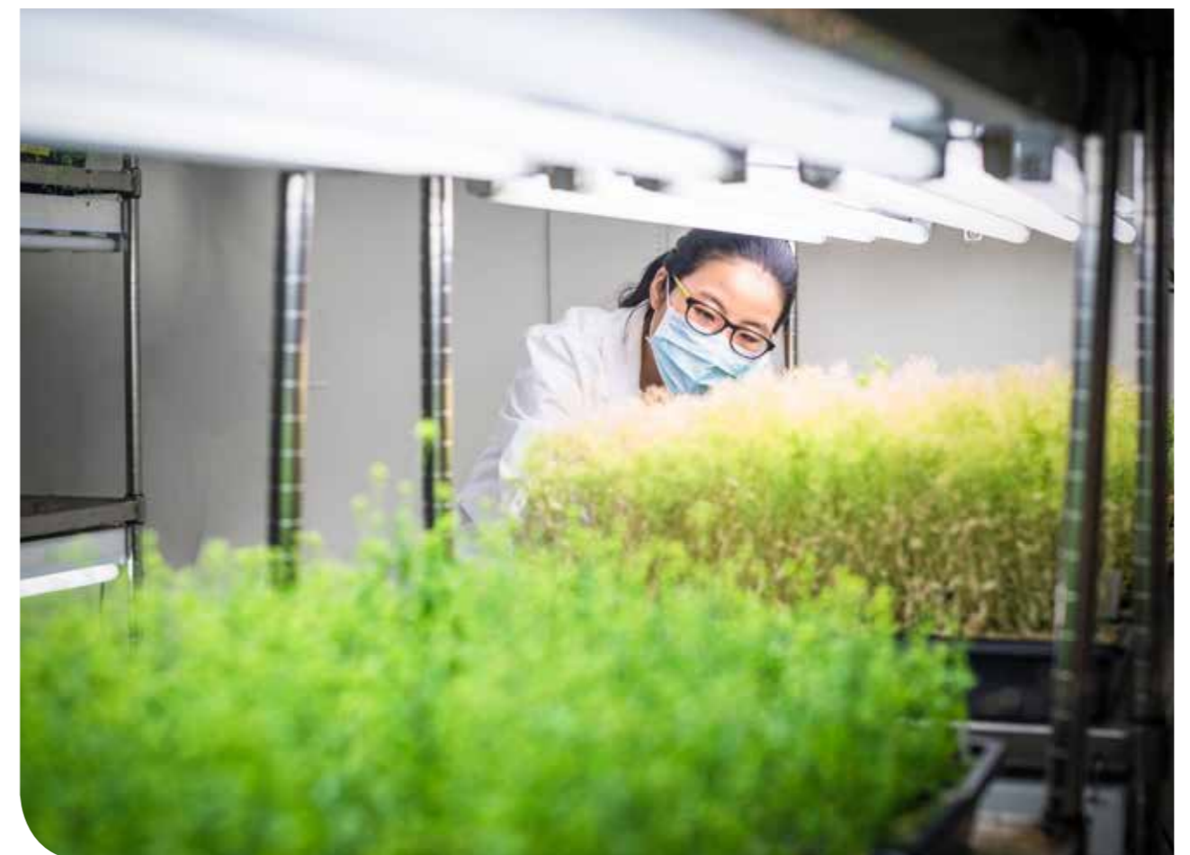
Fitotrone: controlled environment room, temperature and relative humidity adjustment, and photoperiod for quick agronomic screening
